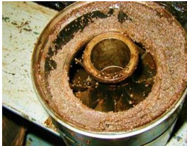
Figure 2. Negative impact of proppant backflow on ESP, clogged with proppant, during the development stage.
