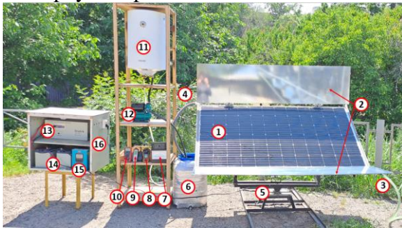
Figure 3. An experimental device based on PVTB of a new dEWHgn
