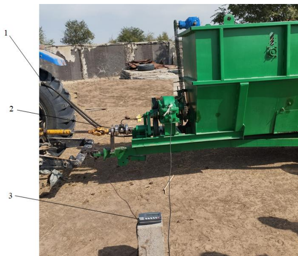
1 – tractor; 2 – strain gauge sensor; 3 – electronic dynamometer
