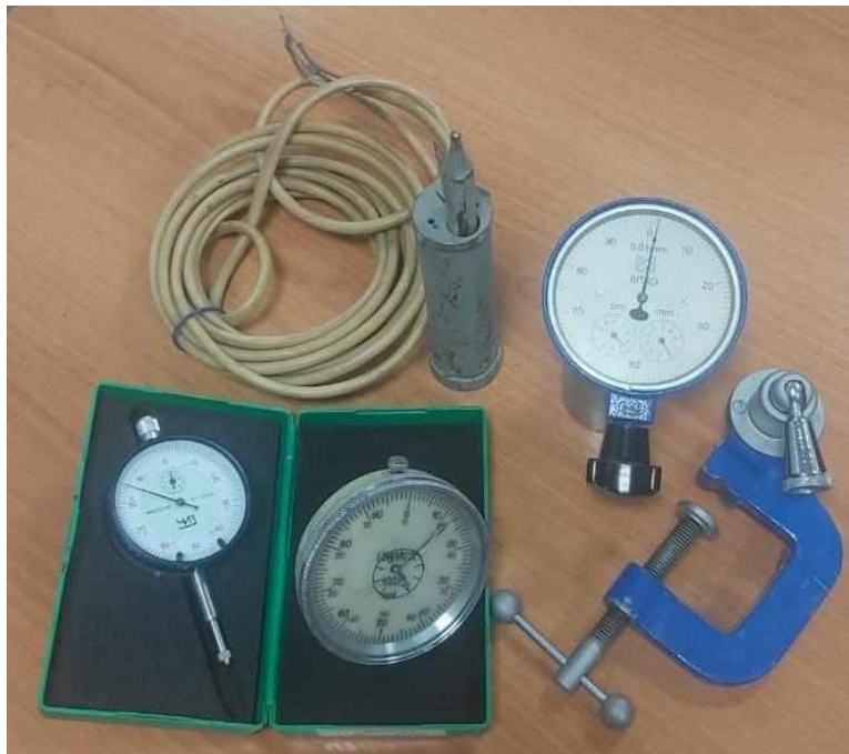
Figure 5. Displacement sensors: clock type indicator ICh-10, deflection gauges of TsNIISK and 6-PAO brands and with a clamp, with an electronic digital displacement sensor on top
