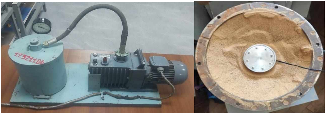
Figure 11. Aerostatic taring tank Left – general view, right – mesdose in the sand tank
